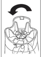
Hold the blades with a cloth. Unscrew the clutch counterclockwise.
