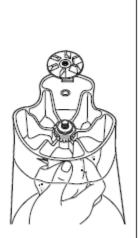
Remove the clutch and felt washer.
