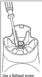
Use a flathead screwdriver to flatten the tabs on the tab washer.
